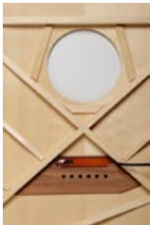
Steel string at bridge plate
